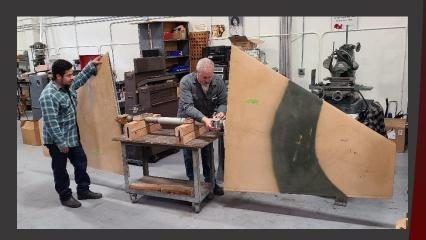
F-5 Horizontal Stabilizers Overhaul/Repair
